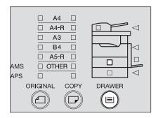
Press the [COPY] button several times until the [OTHER] lamp is lit. "Fxx" appears in the LED display. (Two digits come at "xx".)
